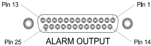
Figure 8. IQ Power BPS Power Supply Alarm Output Connections
