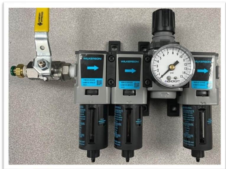
Example Compressed Air Filtration
