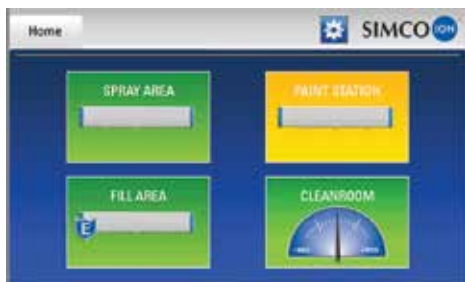
The Home screen displays icons for each device. Icon color represents device status. For Example, four various devices are connected.
