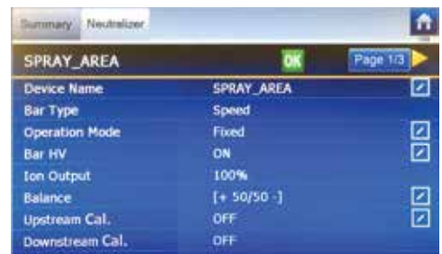
Device screens provide more detailed information such as address, bar/web width, web speed, mounting distance, and run time.
