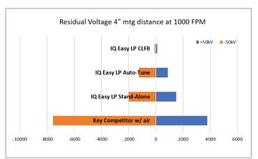
\* Closed-loop Feedback (CLFB) mode requires IQ Easy Modular Sensor Bar and Control Station. \* Auto-Tune mode requires Control Station.
